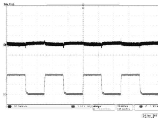
Fig. 9:  $V_{IN} = 1.8V$ ,  $V_{REF} = 0.9V$  source response
