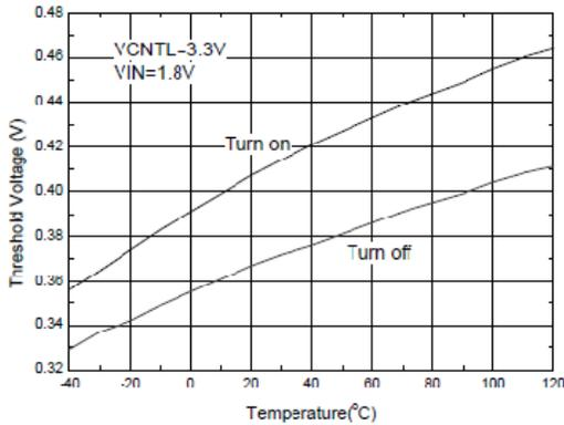
Fig. 4: Turn on and turn off vs. Temperature
