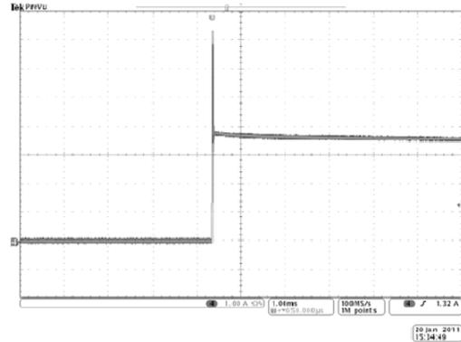
Fig. 14:  $V_{IN}=2.5V$ ,  $V_{REF}=1.25V$  sink short circuit
