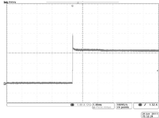
Fig. 12:  $V_{IN}=1.5V$ ,  $V_{REF}=0.75V$  sink short circuit
