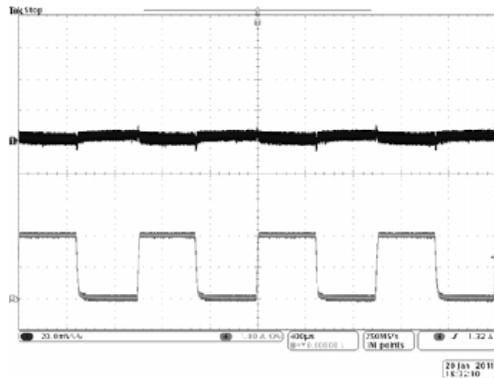
Fig. 8:  $V_{IN} = 1.5V$ ,  $V_{REF} = 0.75V$  source response
