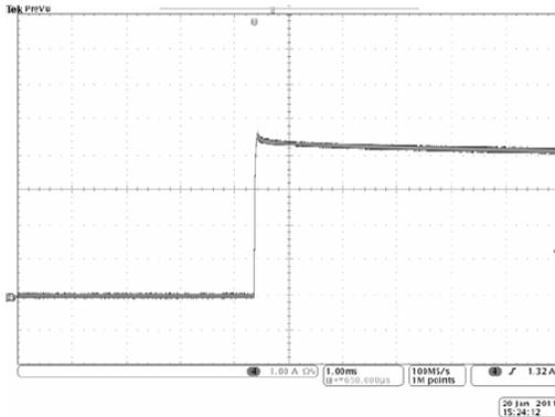
Fig. 11:  $V_{IN}=2.5V$ ,  $V_{REF}=1.25V$  source short circuit
