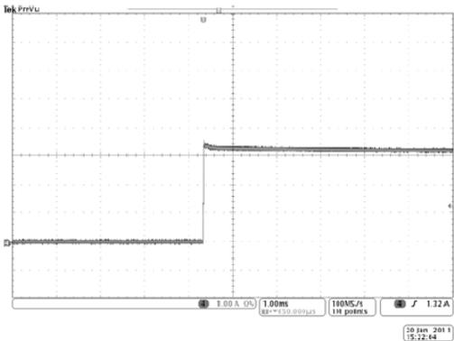
Fig. 14:  $V_{IN}=1.5V$ ,  $V_{REF}=0.75V$  source short circuit
