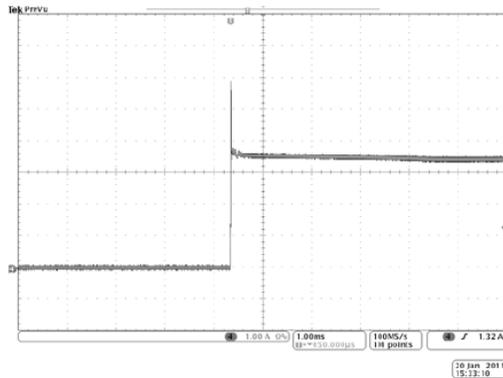
Fig. 13:  $V_{IN}=1.8V$ ,  $V_{REF}=0.9V$  sink short circuit
